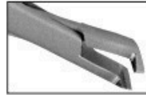
786-1303 Mini with extra long off-set handles T.C distal end cutters with safety hold ● Max. 0.30 mm to 0.50 mm (.012" to .020") ■ Max. 0.46 mm to 0.64 mm (.018" to .025") ⊗ Max. 0.38 mm to 0.53 mm (.0155" to .0215") ⊗ Max. 0.53 mm to 0.64 mm (.021" to .025")
